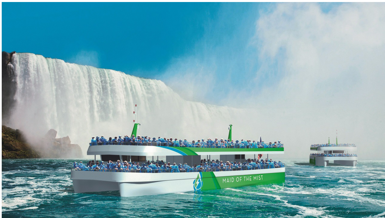
Artist's rendering of the two new all-electric Maid of the Mist tour boats. The boats' design is modular. The modules were built in a shipyard then trucked to site, where they were craned into the assembly area near the river. Craning the vessel modules to the assembly area was challenging due to the difficult topography of the area. The boats' hulls are made from 5086 H116 marine-grade corrosion-resistant aluminum alloy.
